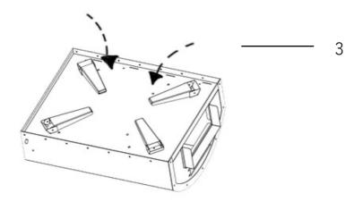
STEP 2: Attach the handle on the Door.
