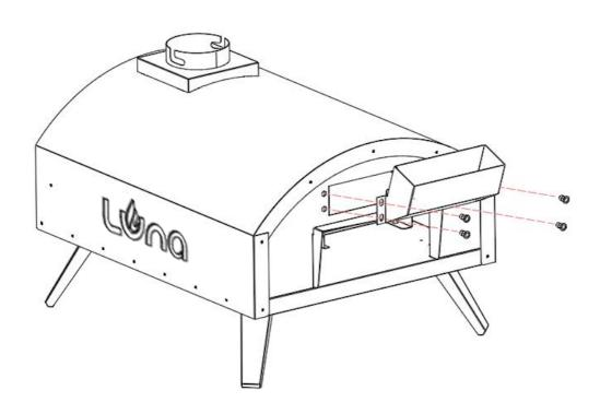
STEP 6: Twist to locate the chimney on the oven body.
