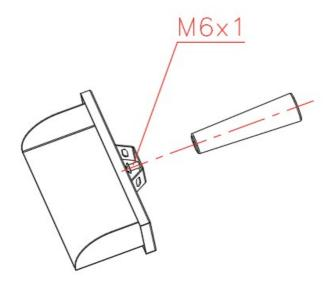
STEP 5 : Attach hopper to the main body using four screws.
